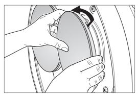
Fig. 7 Grasp the gear edges with your fingers and pull it out of the rubber jigs.
