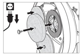
Fig. 10 The sanding pads are also fastened using the plastic plug.
