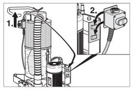
Fig. 19 Hook the on/off switch into the transport support on the motor switchbox.
