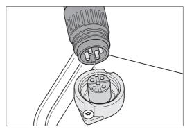
Fig. 21 Make sure that the nose of the plug is inserted into the groove of the socket.
