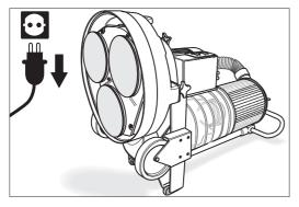
Fig. 34 Tilt the machine backwards to access the sanding gear. Make sure the machine is in a safe position!
