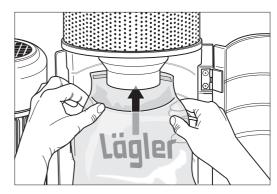
Fig. 16 Make sure the dust bag is in the correct position in the container (print towards you, adhesive strip towards the rear).
