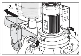
Fig. 45 The chassis can be moved backwards once the crossnut fasteners have been loosened.
