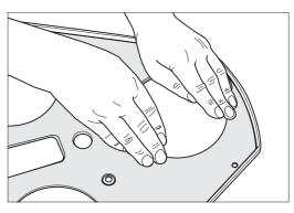
Fig. 56 Press the sealing felt carefully all over, especially at the edges and around the cutaways for the sanding disc gears.
