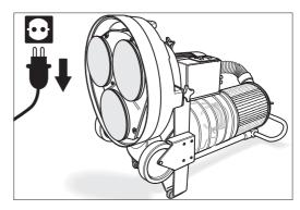
Fig. 3 Carefully tilt the machine backwards to be able to access the gears. Make sure the machine is in a safe position!
