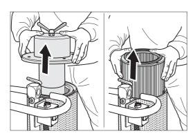
Fig. 28 Remove the cover and remove the filter insert.
