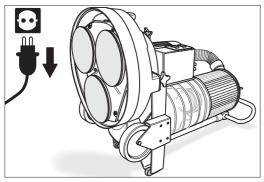
Fig. 52 Carefully tilt the machine backwards to be able to access the gears. Make sure the machine is in a safe position!
