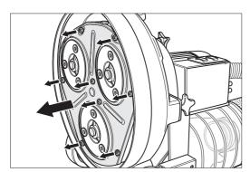
Fig. 36 Then remove the eight screws and pull off the cover.
