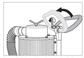
Fig. 2 To tilt the machine, release the clamping lever of the handle first and press the handle forward.
