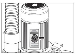
Fig. 58 The seal of approval on the motor indicates when the next maintenance check is due.
