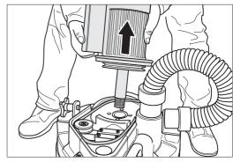
Fig. 48 Lift the motor off the machine casing vertically and remove the V-belt.
