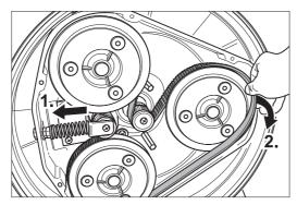
Fig. 39 Push the tooth belt tensioner back and remove the tooth belt.
