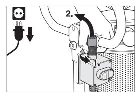
Fig. 43 Loosen the ring nut and remove the cable plug.
