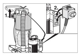
Fig. 44 Hook the on/off switch into the transport holder on the switchbox.
