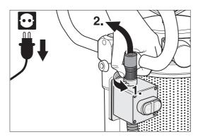
Fig. 18 Loose the ring nut and remove the plug from the mains.
