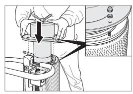
Fig. 31 Replace the cover and **loosely** replace the cap
