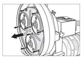
Fig. 54 Then remove the eight screws and pull off the
