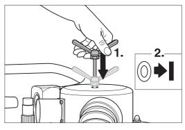
Fig. 23 Push the cleaning slide as deep as possible into the filter unit (1.). Then you can turn the machine back on again (2.).
