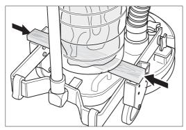
Fig. 26 Place a board between the closed dust bag box and the chassis.
