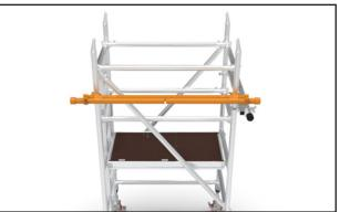
The 2 arms on each stabiliser should be extended such that the rubber caps press firmly against the wall of the lift shaft. Now, tighten the half coupler around the arm to stop retraction. The tower is now held firmly in position.
