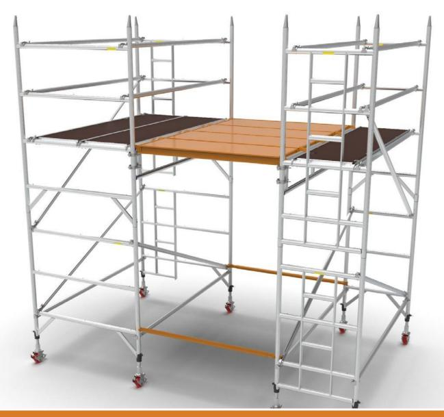
Working from the towers, install four 1.6m horizontal braces as guard rails. Ensure that the braces are hooked onto the frame uprights just above the frame horizontals. Ensure that the braces are hooked on from the inside facing outwards. Any issues with the brace not fitting will be due to the tower not being level. Check the two uprights of the frames are both vertical. Now the 2.4m horizontal braces acting as guard rails on the inside faces of the two towers can be removed (4 total).
