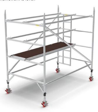
Working from the platform, install a second set of 4 rung frames onto the 1st frames. Then, on the ladder side only, clip a brown diagonal brace onto the 2nd rung down. The other end connects to the 3rd rung below on the opposite frame. Diagonal braces always run parallel to the braces below.
