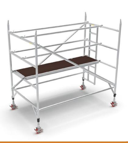
Remove the diagonal brown brace on the non-ladder side of the tower and replace with a 2.4m platform beam. Ensure the top tube of the platform beam is in-line with the top horizontal rungs on the frames and the couplers are fully tightened.
