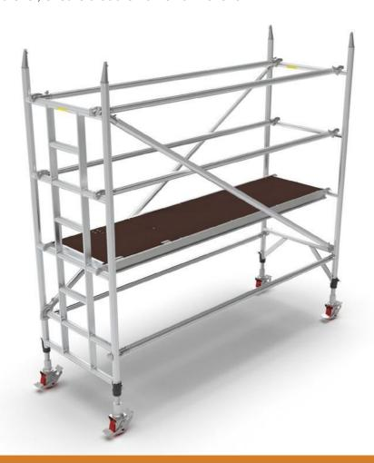
Working from the platform, install a second set of 4 rung frames onto the 1st frames. Then, on one side only, clip a brown diagonal brace onto the 2nd rung down. The other end connects to the 3rd rung below on the opposite frame. Diagonal braces always run parallel to the braces below.
