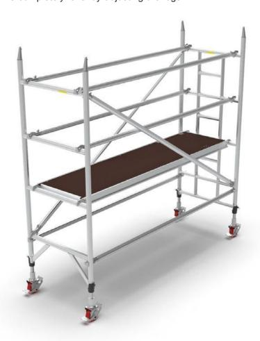
Working from the platform, install a 2 rung main frame & a 2 rung ladder frame onto the 4 rung frames. Then, on one side only, clip onto the top rung 1 more brown diagonal brace. The other end connects to the 3rd rung below on the opposite frame. Diagonal braces always run parallel to the braces below.
