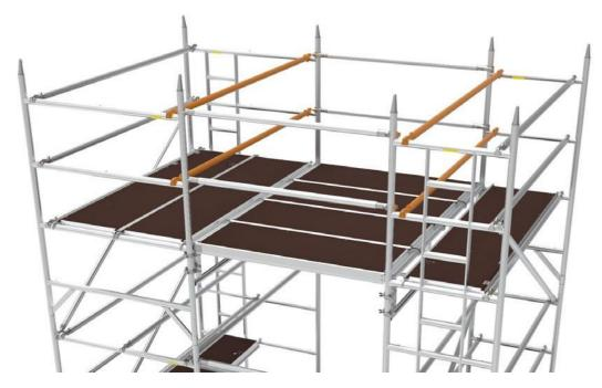
**Step 3**Working from the two towers, unclip the 1.6m guardrails from the bridge sections
