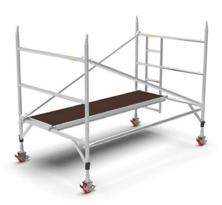
Working from the ground, install a 4 rung main frame & a 4 rung ladder frame onto the 3 rung frames. Then, on the ladder side only, clip a brown diagonal brace onto the 2nd rung down. The other end connects to the 3rd rung below on the opposite frame. Diagonal braces always run parallel to the braces below.
