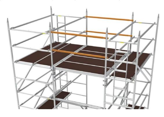
**Step 4**Next, remove the bridge platforms. Then the horizontal joining braces.
