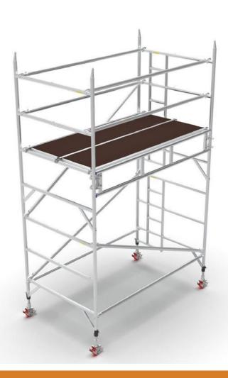
Insert the leg & castor assembly into the base of a S/W 3 rung main frame and S/W 3 rung ladder frame. Ensure the spring loaded pin is engaged into the hole in the side of the frames. Ensure all 4 wheels have the brakes applied.
