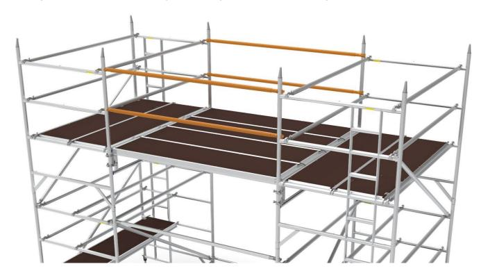
**Step 4**Next, remove the bridge platforms. Then the horizontal joining braces.
