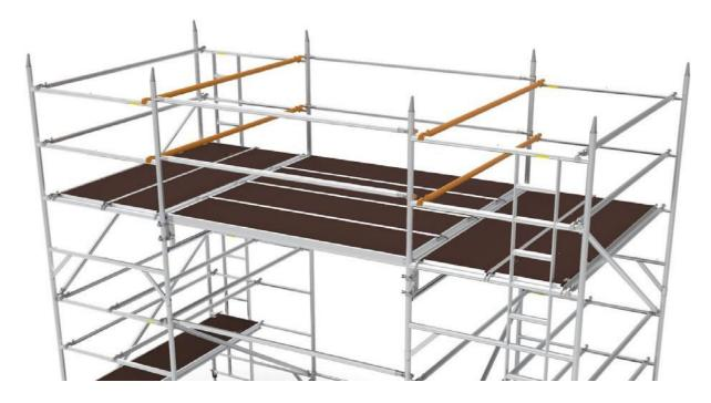
**Step 3**Working from the two towers, unclip the 2.4m guardrails from the bridge sections
